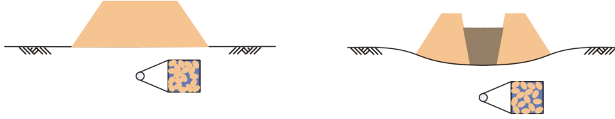
Figure 5.9: Liquefaction phenomena below a dam under a high cycle loading
